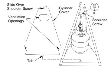
Figure 13 - Installing Cylinder Cover
